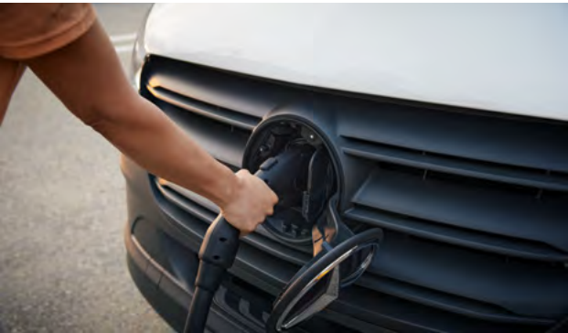
CCS rapid charging port, 115kW max. capacity.
